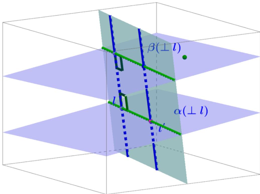
Two planes perpendicular to a straight line are parallel to each other.
