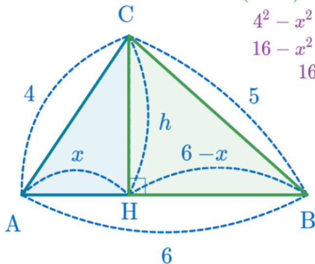
$$\begin{aligned}x^2 + h^2 &= 4^2 & h^2 &= 4^2 - x^2 \\(6-x)^2 + h^2 &= 5^2 & h^2 &= 5^2 - (6-x)^2 \\4^2 - x^2 &= 5^2 - (6-x)^2 \\16 - x^2 &= 25 - 36 + 12x - x^2 \\16 &= -11 + 12x & 27 &= 12x\end{aligned}$$
