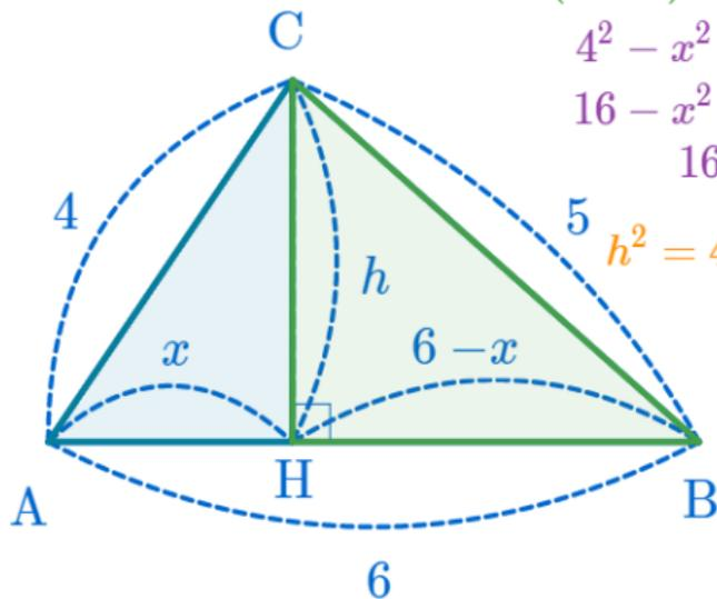
$$\begin{aligned}x^2 + h^2 &= 4^2 & h^2 &= 4^2 - x^2 \\(6 - x)^2 + h^2 &= 5^2 & h^2 &= 5^2 - (6 - x)^2 \\4^2 - x^2 &= 5^2 - (6 - x)^2 & \therefore x &= \frac{9}{4} \\16 - x^2 &= 25 - 36 + 12x - x^2 \\16 &= -11 + 12x & 27 &= 12x & 9 &= 4x \\h^2 &= 4^2 - \left(\frac{9}{4}\right)^2\end{aligned}$$
